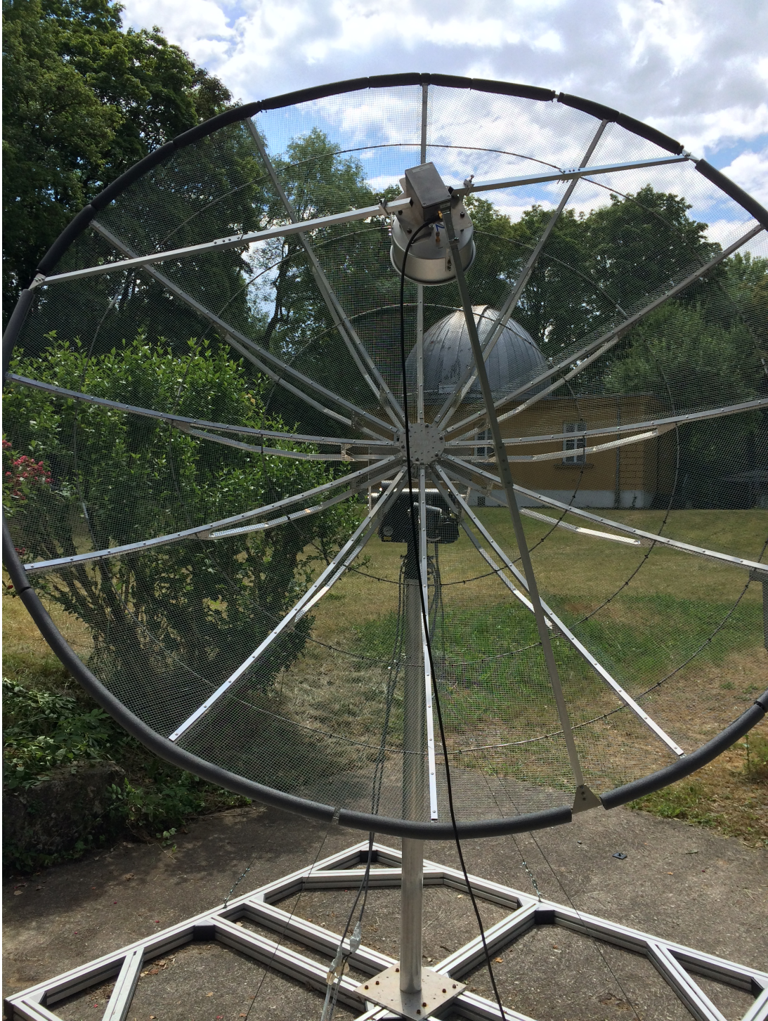
Figure 4.12: The SRT Antenna
